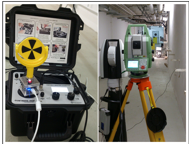
Figure 7. Vibration analysis of a controlled excitation based on acceleration measurements from the PSVC 9210D, video streams from the telescope camera of the Leica MS50, 3D coordinates from the LT Leica AT960-LR and acceleration measurements from the IMU Brick 2.0.
