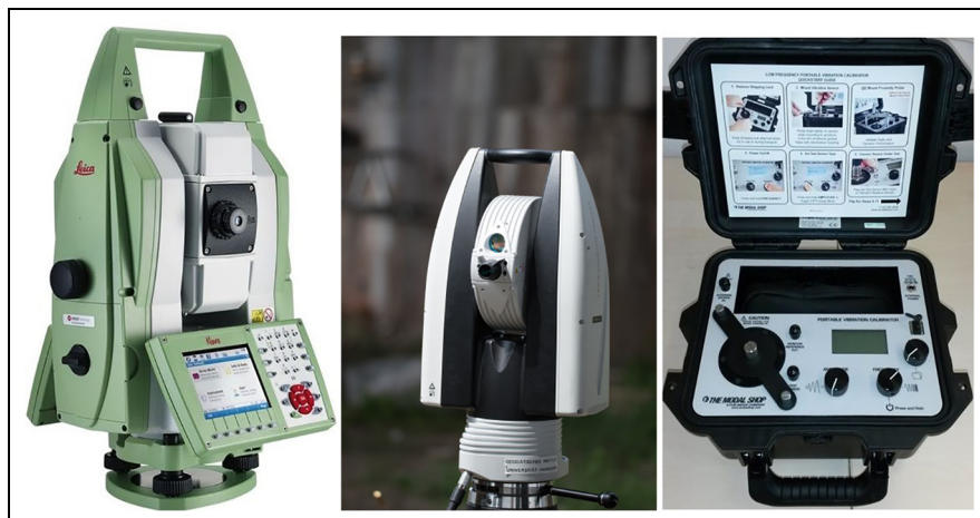
Figure 1. Leica Nova MS50 MultiStation (left), Laser Absolute Tracker AT960-LR (middle) and Portable Shaker Vibration Calibrator 9210D (right).
