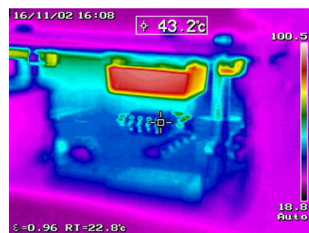
FIGURE 6.17.: Thermography of sympathetic heating in the BCCD. The excess heat of the transistor heats the current measurement amplifier below, thereby causing an additional drift in the current output.
