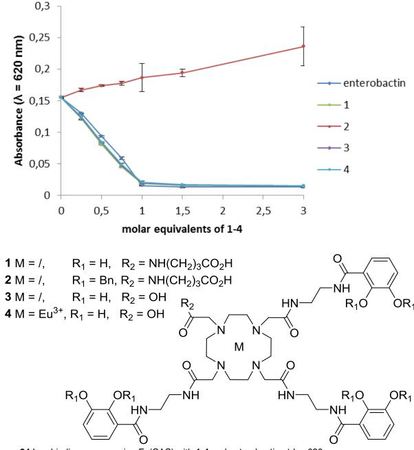
**Figure 24** Iron binding assays using Fe(CAS) with **1-4** and enterobactin at  $\lambda = 620$  nm.
