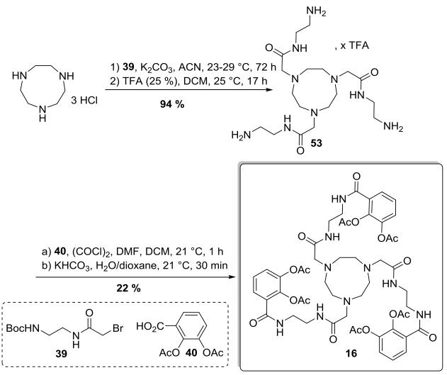
Figure 34 Synthesis of the NOTAM derivative 16.
