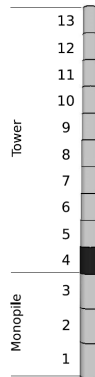
Figure 3.10.: Element numbering of the simulated monopile model. Damage is simulated by a decreased stiffness (10%) of the element marked in black.
