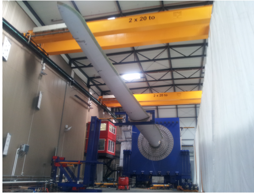
Figure 4.11.: Rotor blade installed in test rig. Load frame connected to blade at 17.5m from blade root [163].
