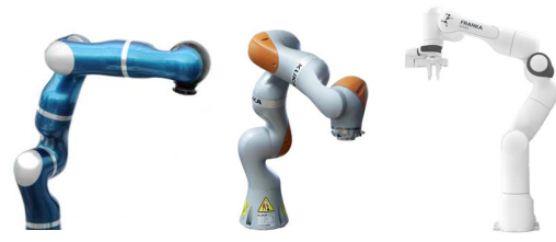
Fig. 2. From left: The DLR LWR-III (by courtesy of DLR), the KUKA LBR iiwa, and FRANKA EMIKA (by courtesy of FRANKA EMIKA GmbH).
