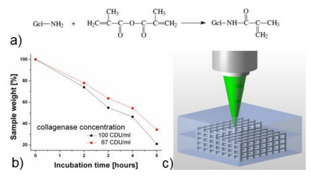
2.2. Scaffold Fabrication Using Two-Photon Polymerization (2PP)
