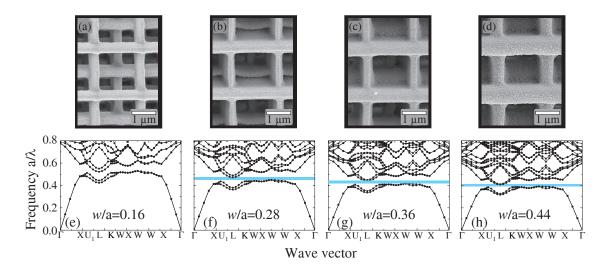
**Figure 5.** (a–d) Woodpile crystals with different filling factors and the photonic band structures (e–h) calculated for materials with the relative permittivity  $\varepsilon=6$  in the air surrounding them. Wave vectors are given for a region of the irreducible Brillouin zone, which includes the edges of the complete photonic band gap. The regions of the complete photonic band gap are marked with blue.
