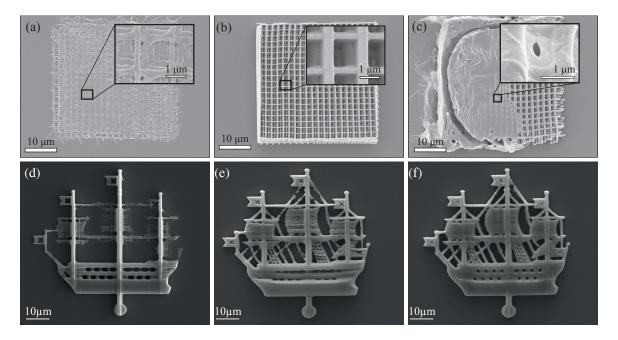
**Figure 2.** Scanning electron microscopy images of woodpile photonic crystals fabricated at: low (a); normal (b) and high (c) exposure; (d–f) scanning electron microscopy images of the wind vane from the top of the Admiralty in Saint Petersburg, Russia, fabricated at different exposures.
