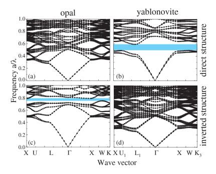
**Figure 4.** Photonic band structure for (a) direct opal; (b) directed yablonovite; (c) inverted opal and (d) inverted yablonovite. The calculations were performed for materials with the relative permittivity  $\varepsilon=13$  in the air surrounding it. Wave vectors are given for a region of the irreducible Brillouin zone, which includes the edges of the complete photonic band gap of the discussed structures. The regions of the complete photonic band gap are marked with blue.
