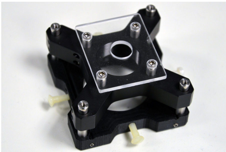
Figure A.3: Applicator attachment to the commercial OCT probe. It was designed as a first attempt to fix the skin for OCT measurements. It was used during first clinical trials and the preclinical study in Chapter 6.
