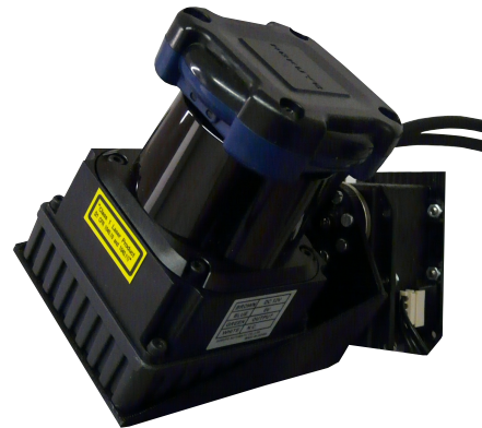
Figure 1. An exemplary setup of an actuated laser scanner. We will use data from this system for our experiments. The laser scanner is a Hokuyo UTM-30LX scanning laser rangefinder that is rotated by a Dynamixel MX-64R robot actuator.
