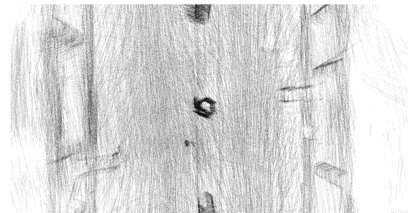
Figure 8. Map generated by the SLAM approach for the metro station dataset using an inappropriate timestamp offset of 19 ms. Blurry edges indicate a small clarity for this point cloud.
