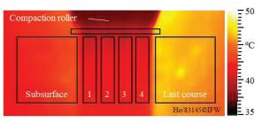
Fig. 2. Thermal process image within the ROI.
