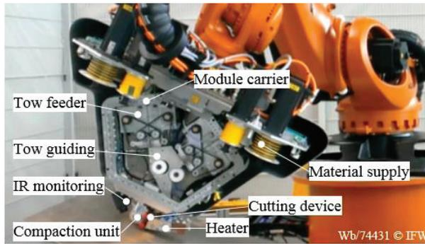
Fig. 1. In-house developed 4 tow automated fiber placement head for robotic applications.
