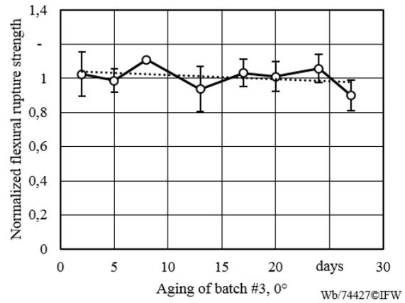
Fig. 5. Normalized flexural rupture strength for batch #3 with 0° fiber direction.
