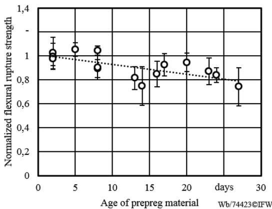
Fig. 9. Normalized flexural rupture strength for 90° specimen as a function of material aging.
