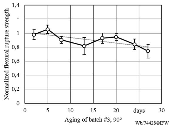
Fig. 7. Normalized flexural rupture strength for batch #3 with 90° fiber direction.
