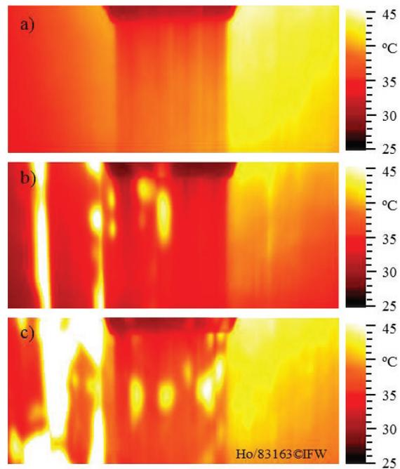
Fig. 3. Thermal images during the lay-up of the third course in the second ply: #3v1 (a), #3v4 (b) and #3v7 (c).
