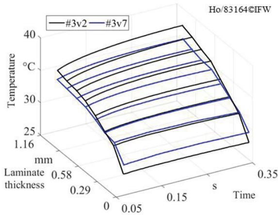
Fig. 4. Comparison of the mean temperature distribution of tow 3 for all plies of experiment #3v2 and #3v7.
