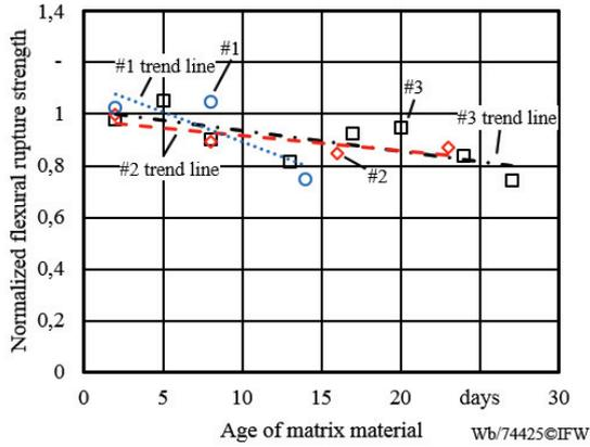
Fig. 8. Normalized flexural rupture strength as a function of aging for test series batches #1 to #3 with 90° fiber direction.
