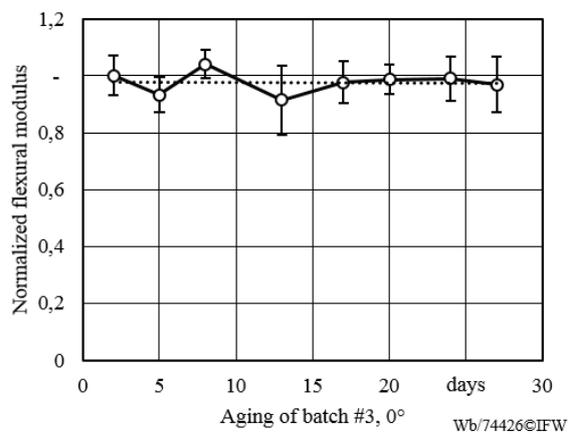
Fig. 6. Normalized flexural modulus for batch #3 with 0° fiber direction.
