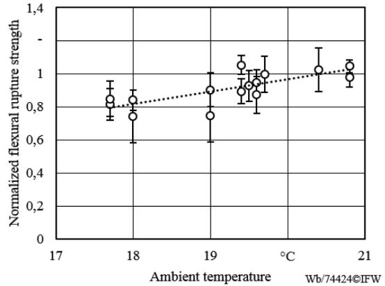
Fig. 10. Normalized flexural rupture strength for 90° fiber direction as a function of ambient-temperature.
