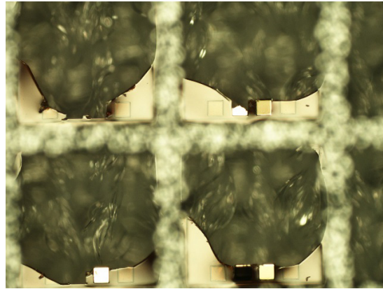
Fig. 7. Remaining silicon grid after the microsystems has been released.
