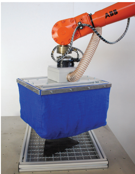
Figure 4 FormHand mounted to a six DOF industrial robot with connected vacuum supply.
