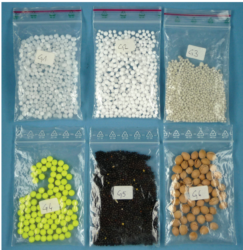
Figure 6 Selection of granules: from top left: EPP, EPS, expanded glass, ABS, rape seeds, cherry pits.
