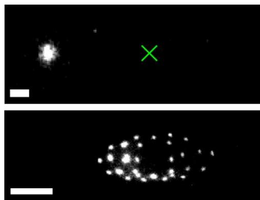
**Figure 1.** Top: A single  $\text{Ar}^{13+}$  ion (position marked by cross) sympathetically cooled by a single laser-cooled  $\text{Be}^+$  ion. White scale bar denotes 20  $\mu\text{m}$ . Bottom: A single  $\text{Ar}^{13+}$  ion sympathetically cooled by several  $\text{Be}^+$  ions. White scale bar denotes 100  $\mu\text{m}$ .
