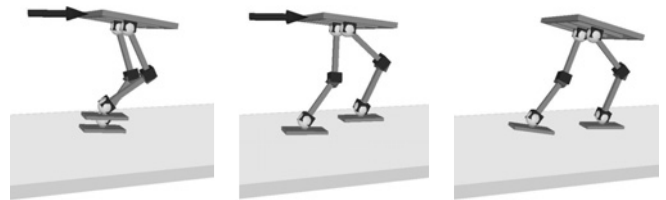
Fig. 13. Unstable situation caused by an impulse to the back of the robot’s torso.
