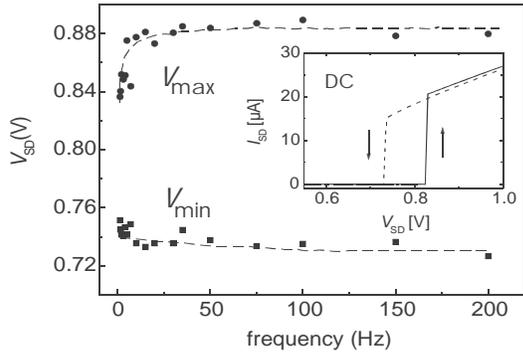
**FIGURE 1.** Hysteresis limits  $V_{\min}$  and  $V_{\max}$  vs. frequency. Inset:  $I$ - $V$  curve at DC.
