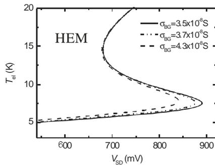
**FIGURE 2.** Breakdown hysteresis for various  $\sigma_{BG}$  (calculated with HEM, see text).
