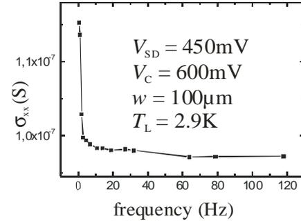
**FIGURE 3.** Subcritical conductivity  $\sigma_{xx}$  vs. frequency (measured values).
