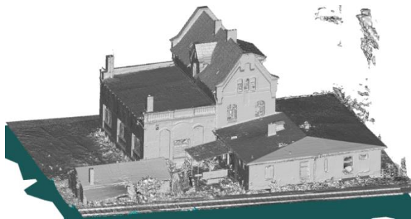
Figure 15. Meshed surface of the building, generated from UAV images, solely. A precise, homogeneous and complete reconstruction could be achieved with the well distributed images of our flight planning and execution concept.
