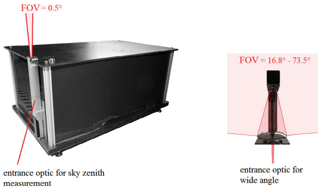
Figure 7. Left: Prototype of the 4D Imager equipped with an entrance optic for sky zenith measurements with a FOV of 0.5^\circ . Right: Entrance optic for a wide angle FOV of 16.8^\circ - 73.5^\circ . This optic can be mounted on the entrance optic for sky zenith measurements.
