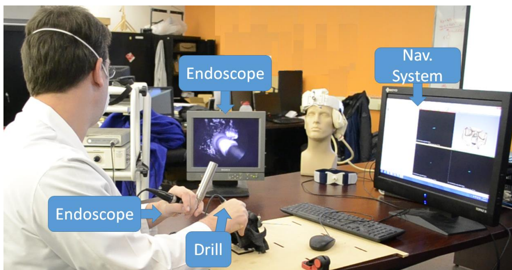
Figure 7. Experimental setup for the drilling experiment evaluating the effects of registration error on the surgeon.
