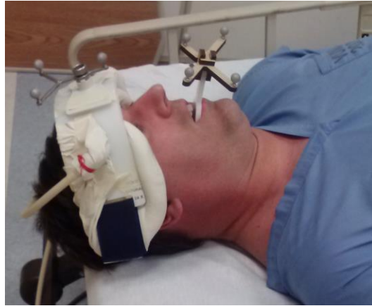
Figure 6. Illustration of the bite block and GJH attached to the subject's head before the simulated bumps were applied. The Brainlab headband is shown in Figure 2.
