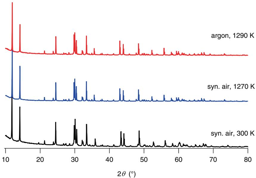
**Figure 1:** *In situ* XRD patterns of  $\text{Na}_2\text{Ti}_6\text{O}_{13}$  in synthetic air and argon. Measurements in both atmospheres show no phase change or additional reflections over the complete temperature range.
