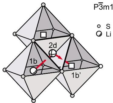
FIG. 11. (Color online) Li diffusion pathway in  $h$ -Li<sub>0.7</sub>TiS<sub>2</sub> as probed by <sup>7</sup>Li spin-alignment echo NMR ( $1b \rightarrow 2d \rightarrow 1b'$ ). The involvement of tetrahedral sites ( $2d$ ) in the Li<sup>+</sup> jump process is energetically favored compared to direct hopping between the (electrically equivalent) octahedral sites  $1b$ . Squares denote vacant Li positions.
