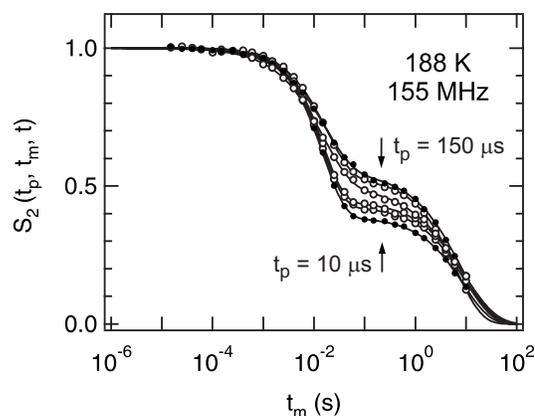
FIG. 4. sin-sin two-time correlation functions  $S_2$  of  $h$ -Li<sub>0.7</sub>TiS<sub>2</sub> for different evolution times  $t_p$  from 10 to  $150 \mu\text{s}$  and constant mixing time of  $t_m = 10 \mu\text{s}$ . Data were recorded at 188 K and 155 MHz. The decay constants  $\tau_{\text{SAE}}^{-1}$  and  $T_{1\text{SAE}}^{-1}$ , characterizing the first and second decay steps, respectively, are independent of  $t_p$ .
