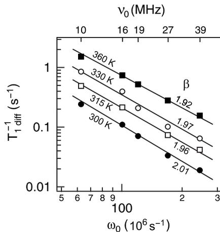
FIG. 9. Frequency dependence (low-temperature flank) of the diffusion induced relaxation rate.  $\beta=2$  indicates that  $T_{1\text{diff}}^{-1}$  in  $h\text{-Li}_{0.7}\text{TiS}_2$  follows simple BPP behavior in the case  $\omega_0 \gg \tau^{-1}$ . Relaxation rates were recorded at various temperatures in the range  $\omega_0 \tau \gg 1$ .
