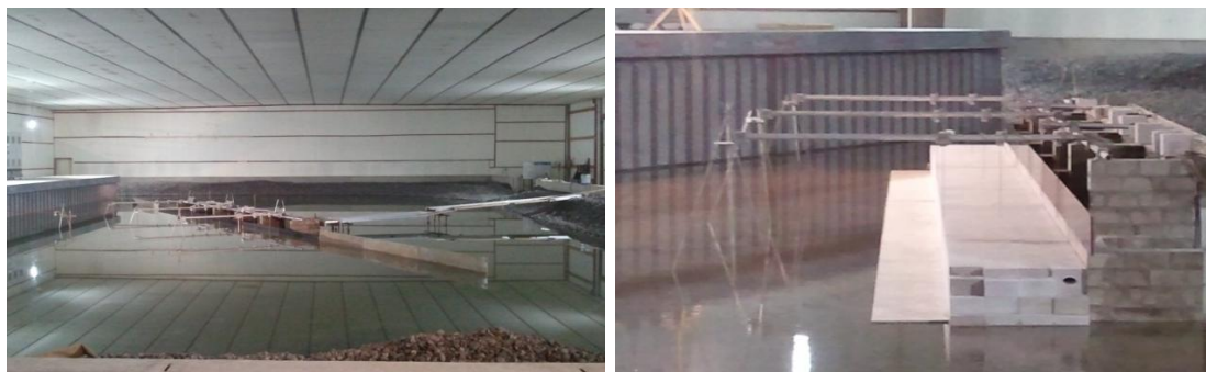
Figure 4. Set-up of Geometry 1 with instrumentation in the 3D wave basin.
