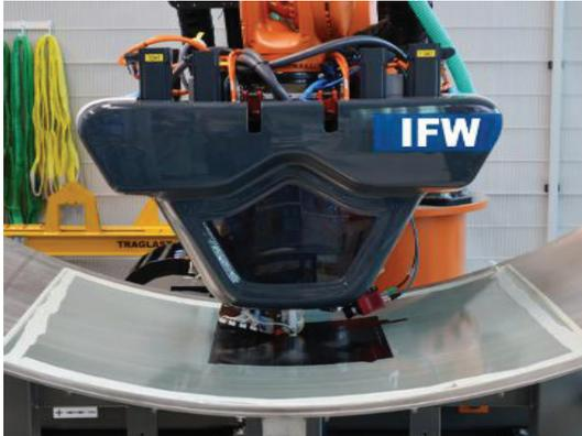
Fig. 3. Laying head with integrated IR camera
