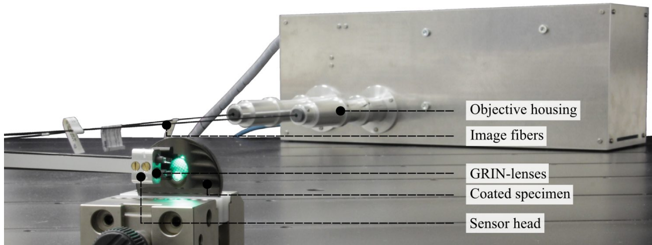
Figure 1. Fiber-optic fringe projection system.
