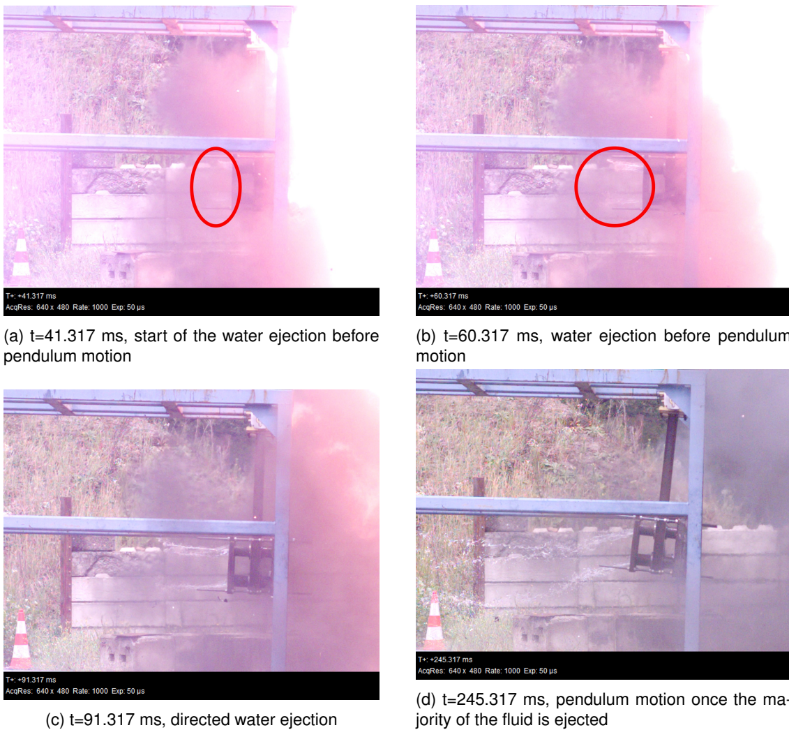
Figure A.45: High speed camera images of the first oscillation of the pendulum for experiment Ta265
