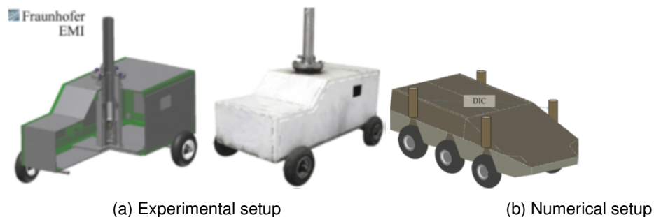
Figure 1.20: Vehicle equipped with a gun type system for dynamic momentum compensation. Taken from [31]
