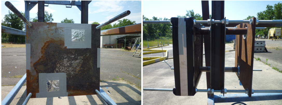
(a) Aluminum foil and tape to seal the tube openings (b) Polystyrene frame for lateral confinement
