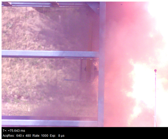
(c) t=75.643 ms, when visualization becomes possible the pendulum has already been set into motion but the water is still situated in between the front and back plate
