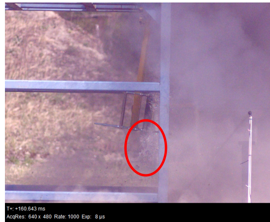
(d) t=160.643 ms, at this time the water ejection becomes notable (circled in red) but the pendulum has already been set into motion before the water ejection can occur
