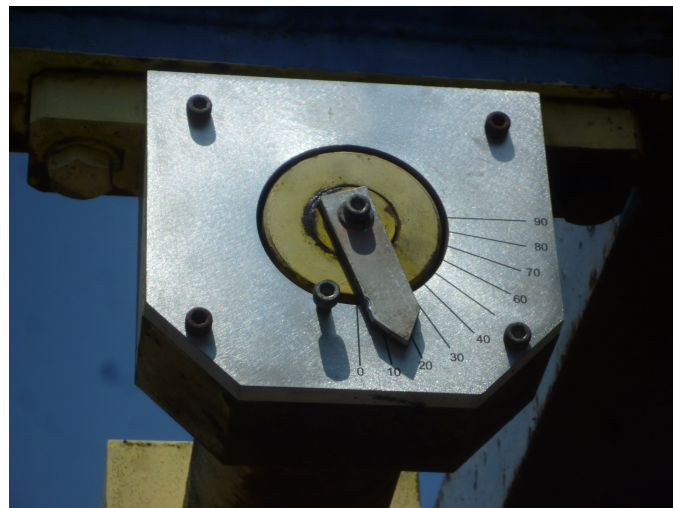
Figure 3.3: Mechanical indicator giving the maximal angle of the pendulum
