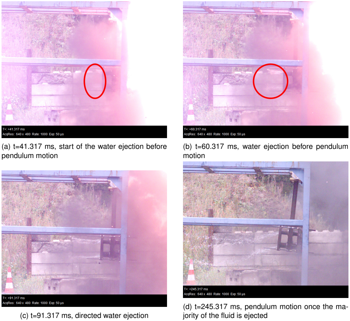
Figure 3.24: High speed camera images of the first oscillation of the pendulum for experiment Ta265
