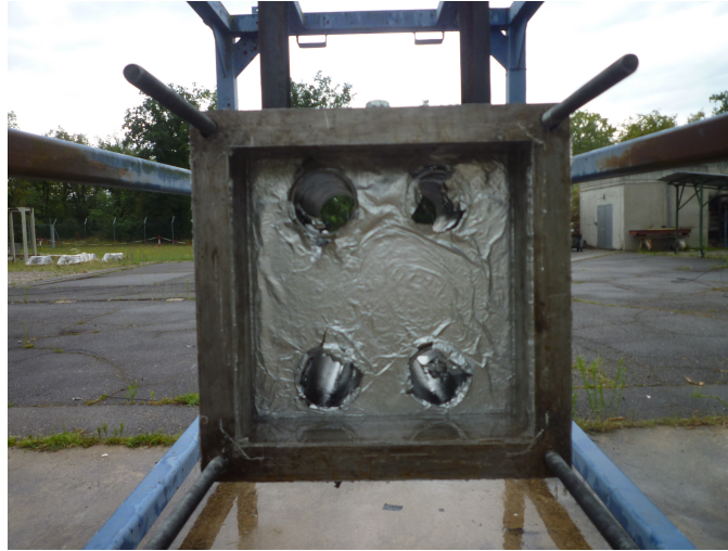
Figure 3.23: Experimental setup with four openings with a diameter of 100 mm for water ejection (front plate not shown)
