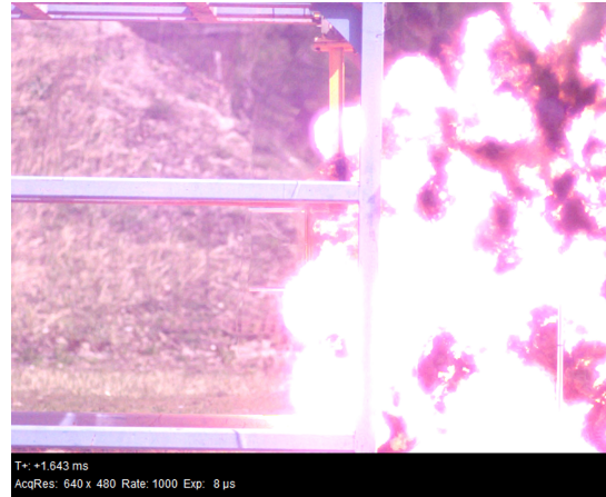
(b) t=1.643 ms, the luminosity of the fireball does not allow to visualize pendulum motion at the start of the experiment
