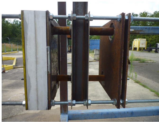
Figure 3.22: Aluminum frame for lateral water confinement
