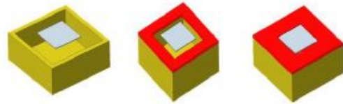
(a) Schematic representation of different water confinement levels. From left to right 0, 50 and 100%.
