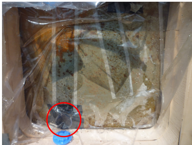
Figure 3.19: Image taken after the experiment. Use of the previously used bags to contain the water. The water bag ruptures towards the front plate, thus covering the entrance of the tubes and preventing water ejection.
