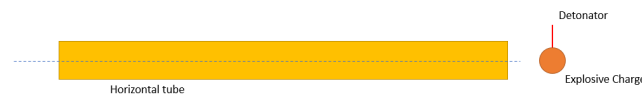
Figure 2.16: Placement of the detonator for the horizontal EDST. Detonator and tube axis perpendicular
