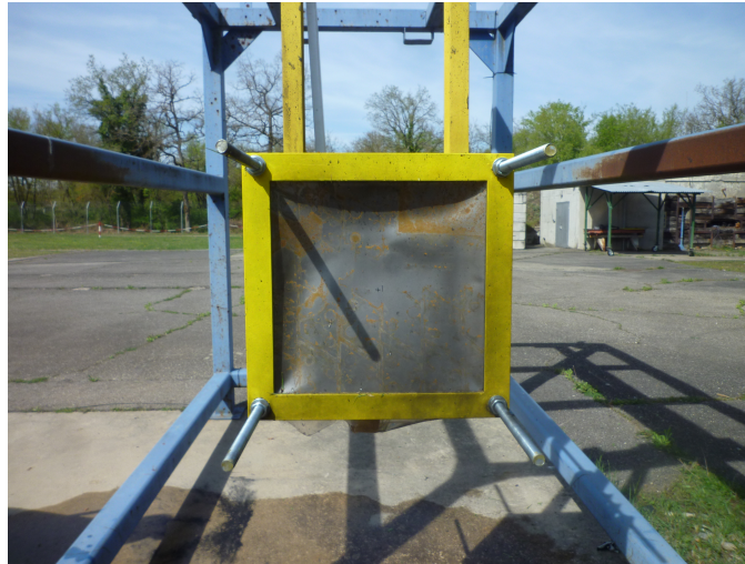
Figure 3.5: Frame for structure rigidity
