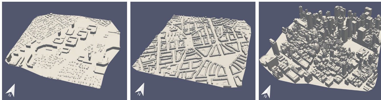
FIGURE 4 Three urban environments we used in this study for the ray tracing of populated areas with different building densities and geometries. The left image shows a mixed district in the city of Berlin (Germany) with single-family houses but also some high-density apartment buildings (Environment A). The center image shows a densely populated district in the city of Hannover (Germany) with largely apartment buildings (Environment B). The right image shows a densely built-up area with high-rise buildings (Environment C) in the city of New York City (United States). All excerpts have an edge length of approximately 1 km.
