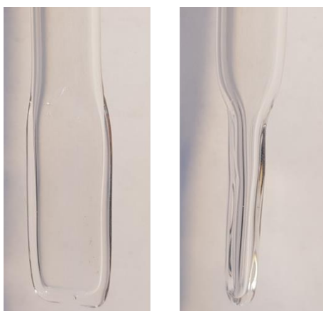
Figure S4: Photographs of the measurement cell for the photocatalytic experiments. The glass vial is pressed to have an inner thickness of less than 2 mm to ensure the illumination of the whole hydrogel.
