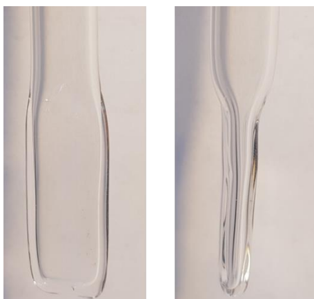
Figure S6: Photographs of the measurement cell for the photocatalytic experiments. The glass vial is pressed to have a thickness of less than 2 mm to ensure the illumination of the whole hydrogel.
