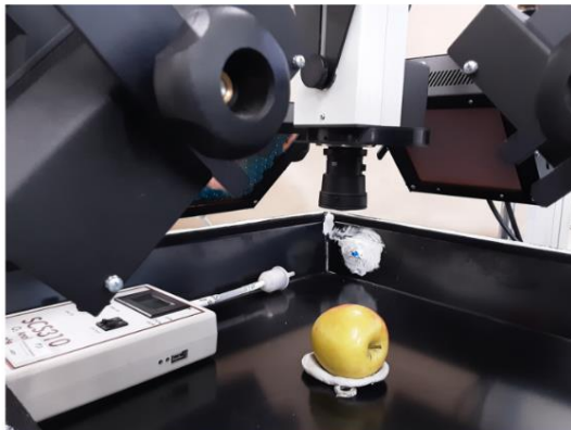
Fig. 1. The structure of the setup: The FluorCAM with four LED panels, CCD camera and apple fruit. The oxygen analyzer's shown at the bottom left side. The box was closed with an acrylic plate (not shown).
