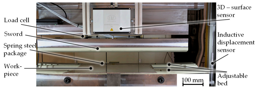
Figure 6. Experimental setup of the scaled Deharde Polygon Forming ® process with extended measuring technology.
