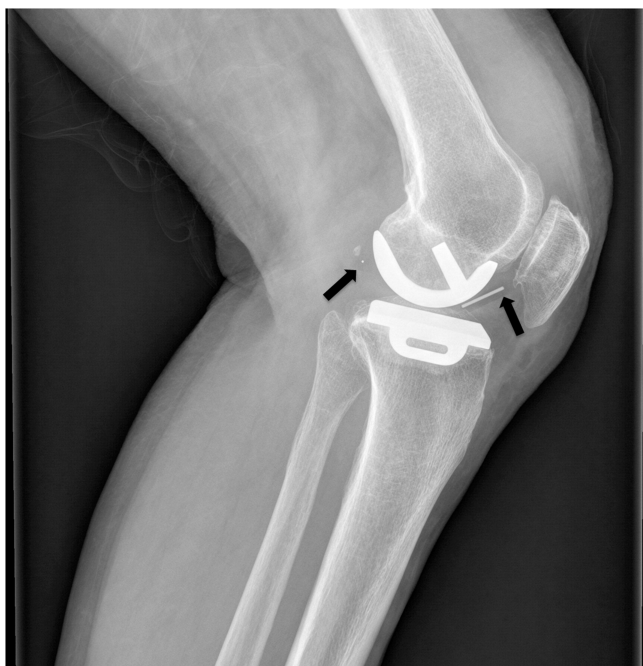
Figure 4. Anterior marker wire and posterior ball marker (shown with black arrows) enabled determination of fracture of this UHMWPE bearing. Reproduced with permission from ref 62. Copyright 2013 Elsevier.
