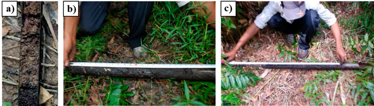
Figure 4. Present status of a layer of humus decomposing from vegetation on the peat layer (a), peat layer with a thickness of 50 cm (b), and 1.2 m (c).
