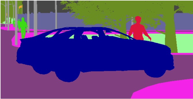
Fig. 2. Synthetic semantic segmentation showing the vulnerability (red/green) of occluded pedestrians on the sidewalk (pink) and on the road (purple)
