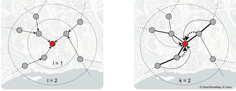
Fig. 2. Left: Graph convolution with two layers, aggregating each node with equal importance. Right: Our proposed approach of aggregating nodes based on traffic flow and hop distance for a maximum hop distance of two.
