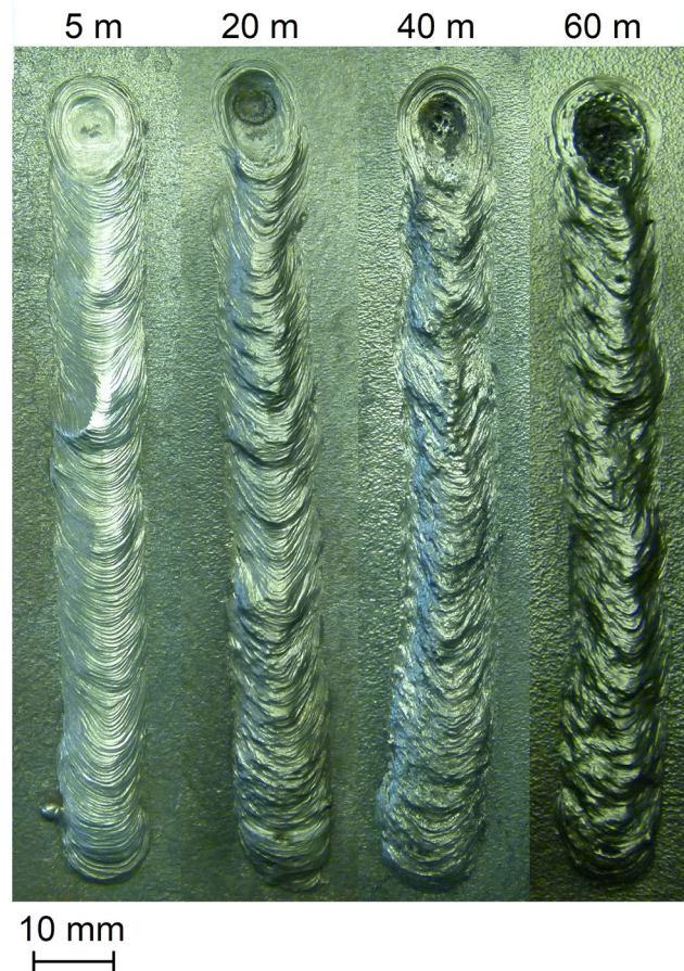
Fig. 10 Bead on plate weld seams welded with the stick electrode HK3 in the water depth 5 m, 20 m, 40 m, and 60 m. The parameters used are listed in Table 2
