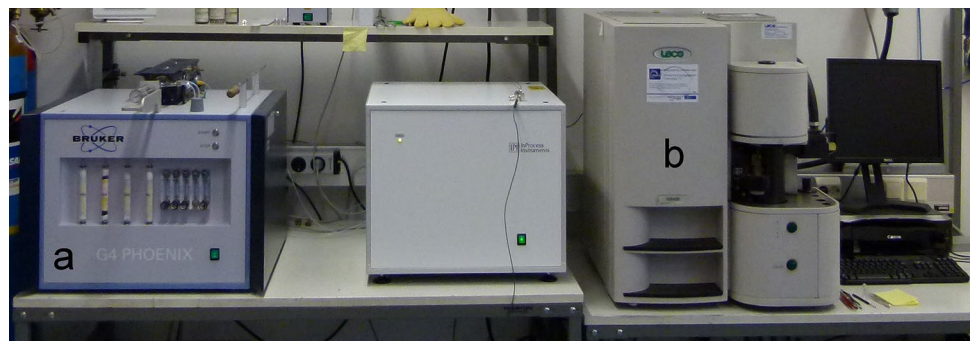
Fig. 2 The Hydrogen analysers used: a Bruker G4 Phoenix analyser for diffusible Hydrogen, b LECO TCH 600 analyser for hydrogen, nitrogen and oxygen
