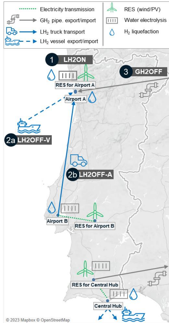
Figure 6.2: Exemplary LH 2 supply pathways shown for an Airport A; 1 – LH 2 on-site supply at/close to the airport, 2a- LH 2 off-site import via vessels, 2b – LH 2 off-site import via road from a neighboring Airport B, 3 – GH 2 off-site import via pipelines and a LFP at the receiving Airport A; export hub perspective shown on bottom of map
