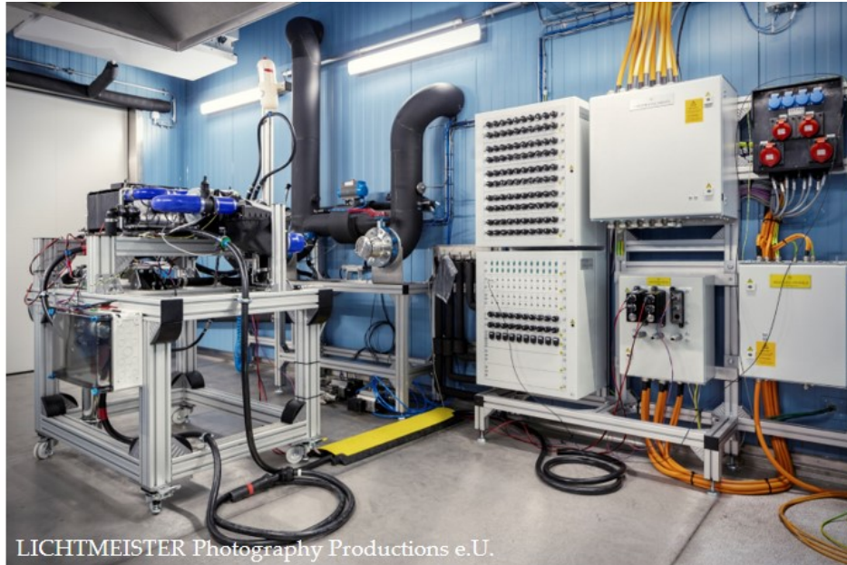
FIG. 4.5 Test rig chamber with experimental fuel cell system.
