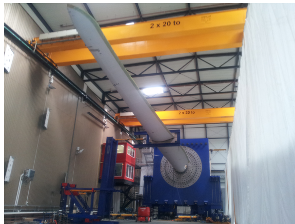
Figure 1. Rotor blade investigated on the test rig [2]
