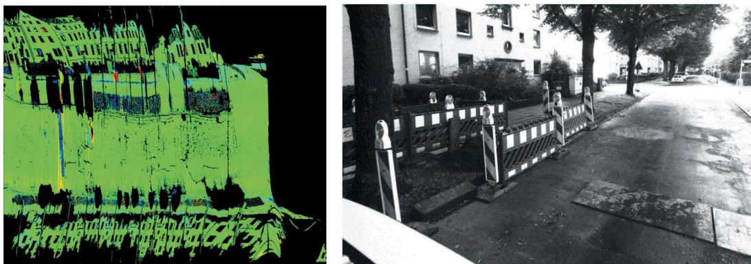
Figure 3. (Left) in red and blue changes can be seen between the images, e.g. the blue stripe on the street stands for an iron slab that was laid in the course of a construction site (right).
