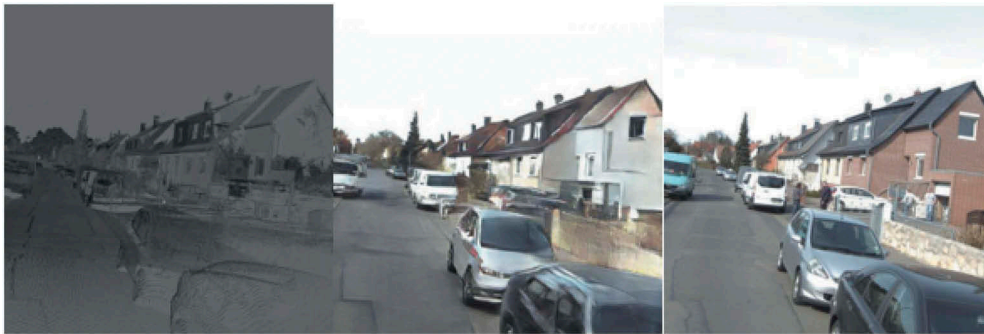
Figure 4. (Left) lidar projection, (right) camera image, (middle) synthesized image.
