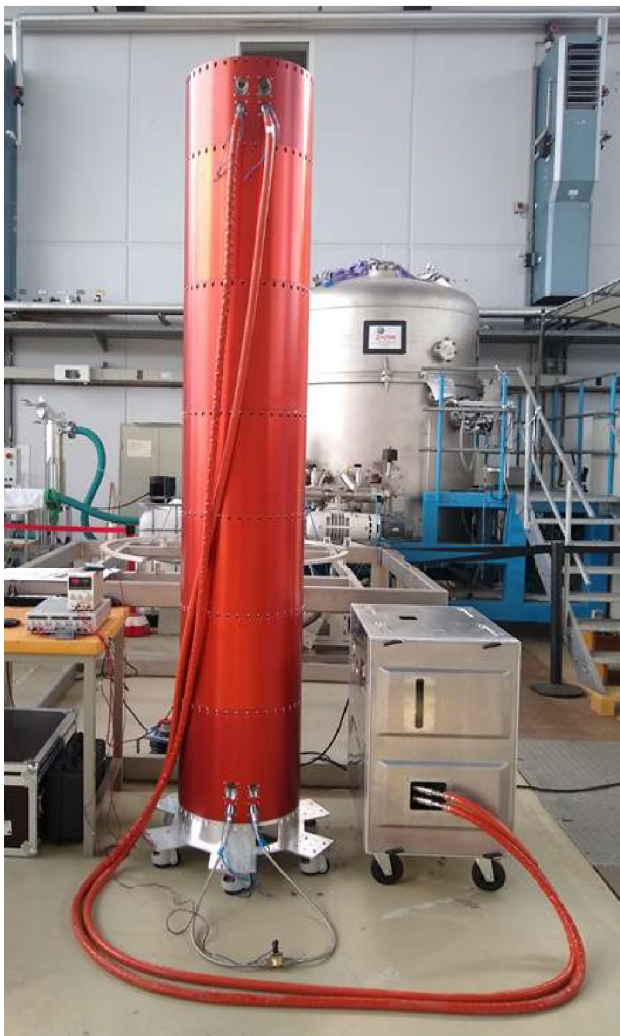
Fig. 6 Flow rate test of the cooling cycles of MAIUS-B. The case which houses the chiller is placed right next to the scientific payload (red hull segments). The orange hoses are equipped with a fire protection to avoid damage during launch. Picture from Elsen (2023)
