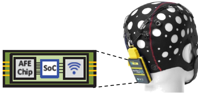
Figure 1.2: The envisioned future BCI system according to [Bel21]. This embedded head-mounted platform is designed to acquire Electroencephalography (EEG) signals, process and analyze brain activity, and send a decision based on the results to an application.
