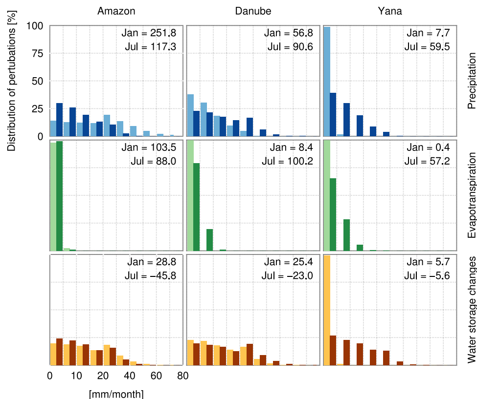
Figure 3. Histograms of 10000 random realizations drawn from a multivariate normal distribution with zero mean and the observation error covariance matrix from (32). The histograms show the distributions of the random perturbations for the three catchments (left column Amazon, (middle column) Danube, and (right column) Yana for (top row) precipitation, (middle row) evapotranspiration, and (bottom row) water storage changes. The left bars (bright colors) correspond to the perturbations of January while the right bars (dark colors) show the perturbations in July. The figure only shows the absolute value of the perturbations as they are symmetric around zero. The numbers in the top right corner of every histogram are the ensemble mean values of precipitation, evapotranspiration, and water storage changes for January and July, respectively, in mm/month.
