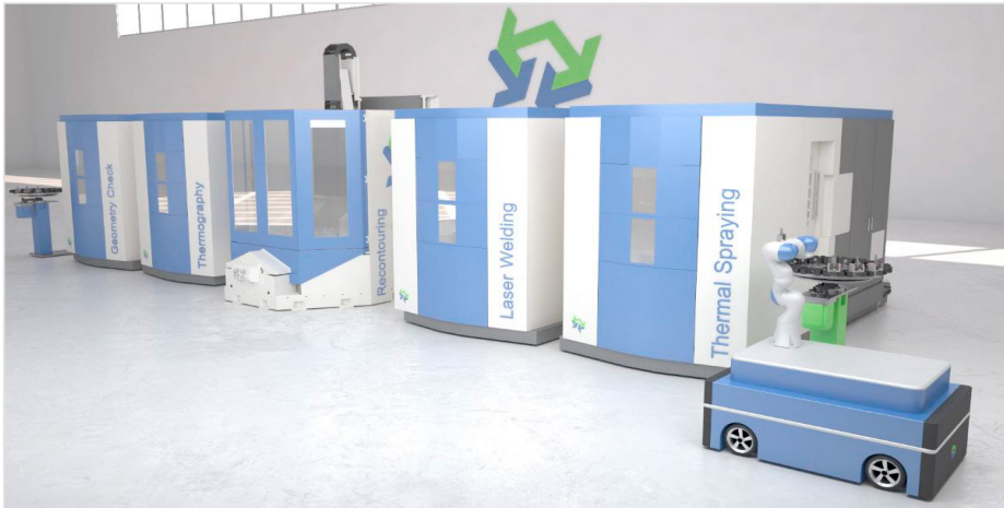
Fig. 2: Schematic arrangement of the included process cells within the demonstrator
