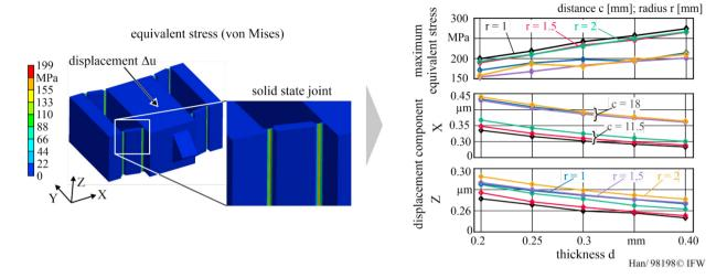
Fig. 6. Equivalent stresses due to the displacement  $\Delta u$  of the piezo actuator.
