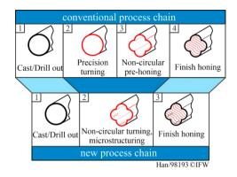
Fig. 2. Conventional and new process chain.
