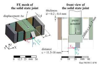
Fig. 5. Solid state joint.
