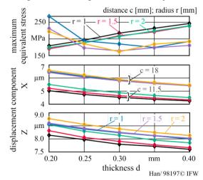
Fig. 7. Displacement of the cutting edge due to process forces.
