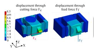
Thereby, the process forces for microstructuring were estimated on the basis of investigations by Kästner [17]. For various materials and similar micro dimple sizes the maximum process force was 10 N. The process forces for turning EN-GJL-250 were only roughly estimated with the specific process forces for a depth of cut of 0.5 mm, a maximum cutting speed of 1,500 m/min and a maximum feed of 0.25 mm.
