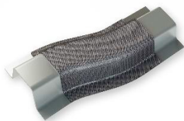
Fig. 1. Hybrid s-rail (high strength steel/organosheet).
