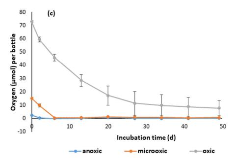
**Figure 4.** (a) Cumulative net N<sub>2</sub>O reduction; (b) cumulative net CO<sub>2</sub> production; and (c) O<sub>2</sub> depletion by strain IGB 4-14<sup>T</sup> under anoxic, microoxic (4% O<sub>2</sub>) and oxic (20% O<sub>2</sub>) conditions. The plotted values are averages of six repetitions, corrected by the average of three controls. Error bars represent the standard deviations. Different letters indicate significant differences (p < 0.05).
