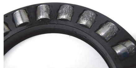
Fig. 10 Significant pittings on the bearing rollers after endurance test (260 h)
