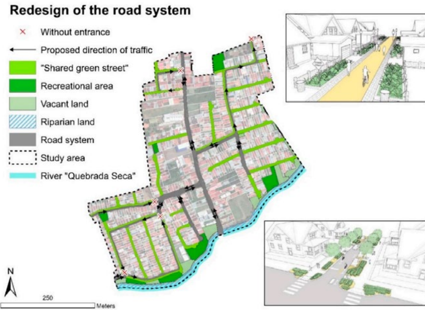
Figure 4.8. Proposal for a redesign of the road system in the RWL to integrate green areas and improve the social dimension of UGI multifunctionality.
