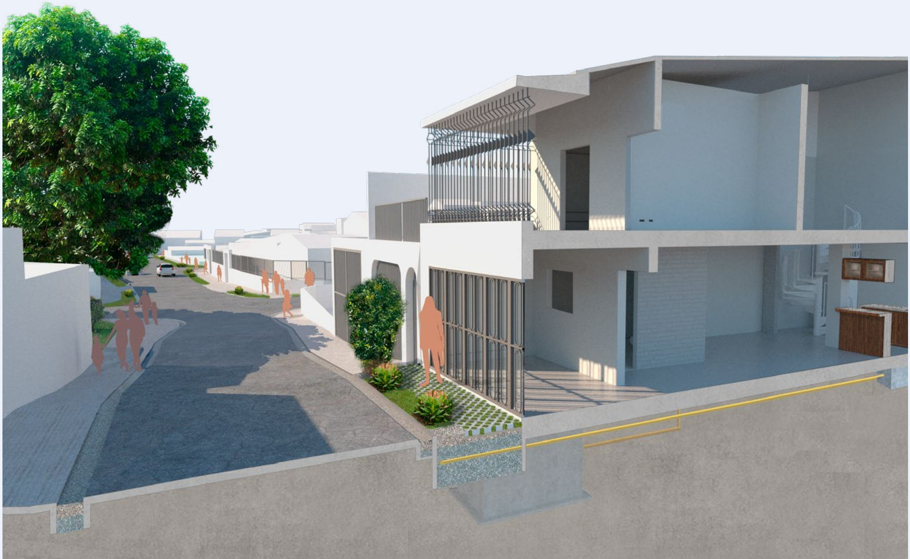
Figure 4.35. Design sketch of the constructed wetland prototype for greywater treatment, integrated into the sidewalk.
