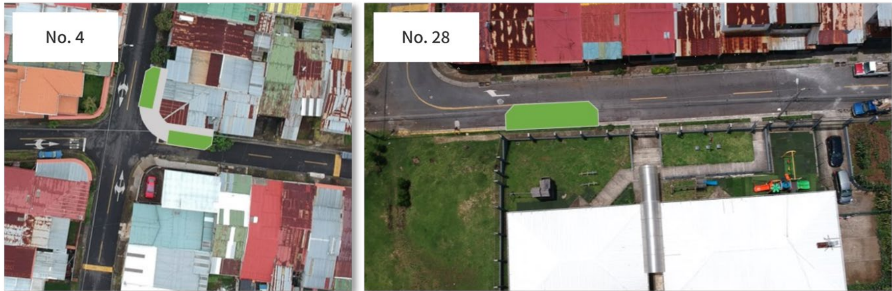
Figure 5.27. Potential placement site and designs for bioretention cells (in green) in the Real-World Lab in accordance with Fluhrer et al., 2021.
