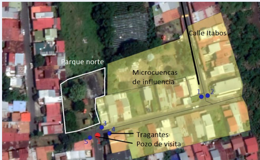
Figure 4.18. Tributary area (in yellow) and location (outlined in white) of the infiltration area prototype.
