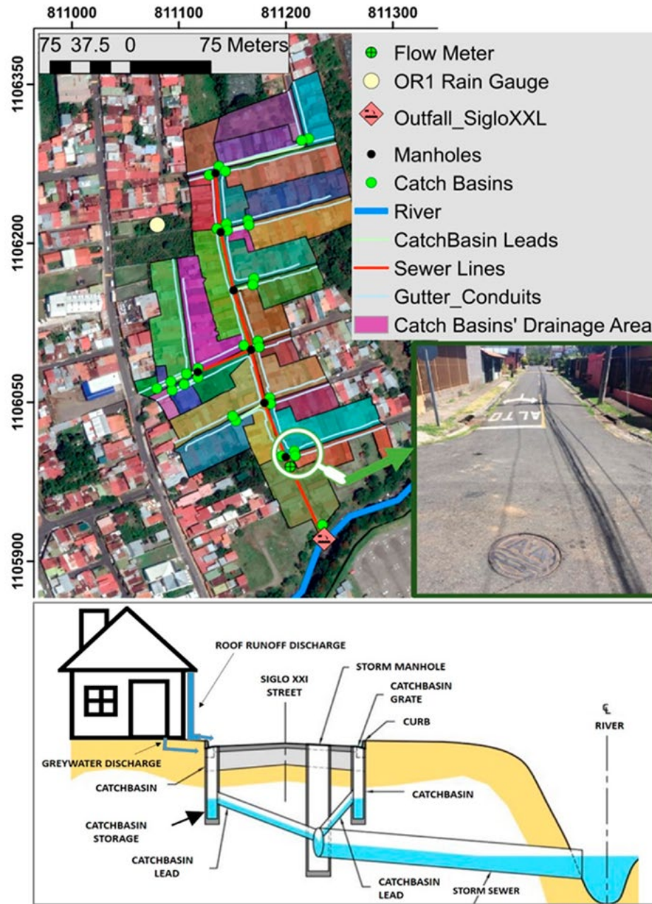
Figure 5.3. Drainage area (top) and schematic representation of hydraulic features (bottom) of the Siglo XXI neighborhood used for rainfall-runoff modeling of the status quo and Nature-based Solutions prototype implementation in the Real-World Lab.
