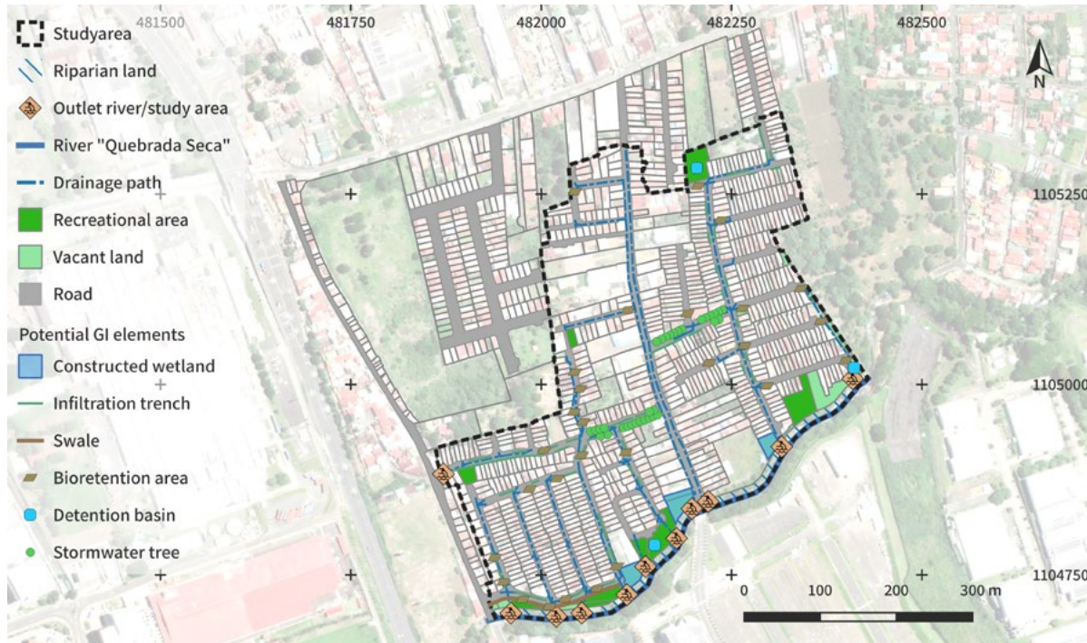
Figure 5.28. Suitable sites for Urban Green Infrastructure placements within the SEE-URBAN-WATER Real-world Lab (Fluhrer et al., 2021).
