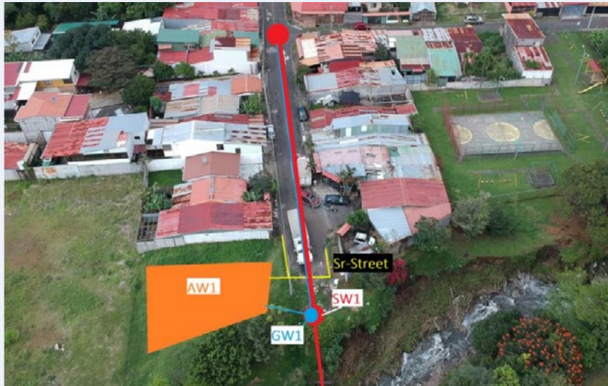
Figure 4.26. Distribution of the proposed storage, conveyance, collection, and treatment systems for the hybrid prototype.
