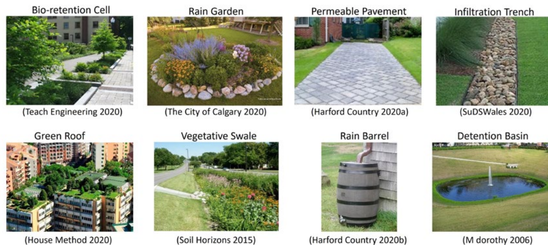
Figure 5.22. Urban Green Infrastructure elements analyzed with regard to their hydrological, social and ecological benefits (Milagres, 2020).
