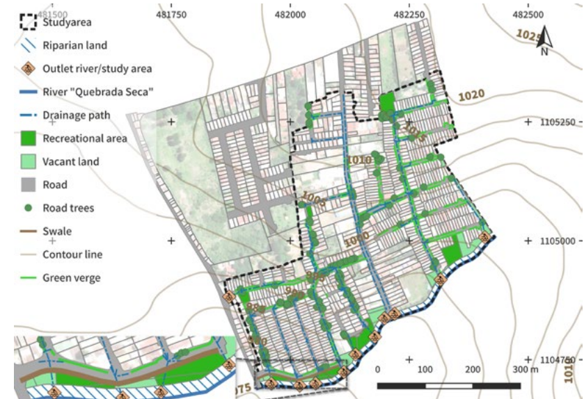
Figure 5.26. Potential placement sites for vegetative swales in the Real-World Lab (Fluhrer et al., 2021).
