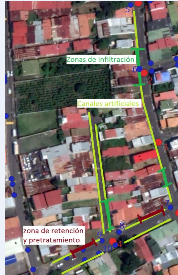
Figure 4.22. Tributary area of the bioretention area prototype.
