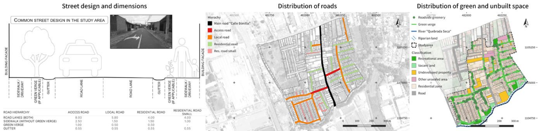
Figure 5.11. Landscape characteristics considered as constraints to a realistic implementation of Urban Green Infrastructure elements: Street design and dimensions of different-hierarchy roads (left), spatial distribution of road hierarchy (middle) and existing green network and available open space (right) for Urban Green Infrastructure in the representative neighborhood (Fluhrer et al. 2021).
