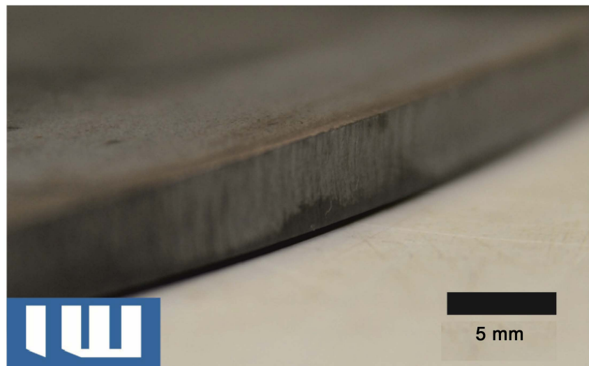
Figure 5. Bottom side of cut edge, S1100QL, 5.3 mm [8]. Only minimal excess material adheres to the bottom edge. The surface is smooth with a bevel angle of 2.1°. This bevel angle serves as an ideal weld preparation for the NVEB welding process, enabling safe penetration of the electron beam, good outgassing characteristics and subsequently high welding speed with comparably low heat input.
