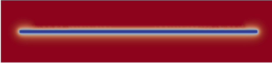
Figure 5.6: Visualization of the nonsmooth phase-field solution of the two dimensional Sneddon test with h = 0.011 and Case 4 . Red represents the fully intact part of the domain, blue the fully broken part and white stands for the transition zone. Reprinted from [93] with permission of Elsevier.
