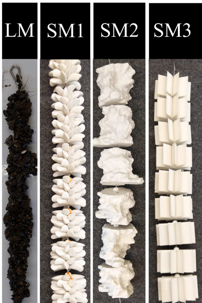
Fig. 3. Live mussel dropper line (LM) next to surrogate mussel dropper line 1 (SM 1), surrogate mussel dropper line 2 (SM 2) and surrogate mussel dropper lines 3 (SM 3).
